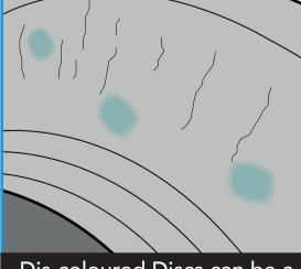
Dis-coloured Discs can be a sign of heat damage caused by Sliding or Adjustment issues
