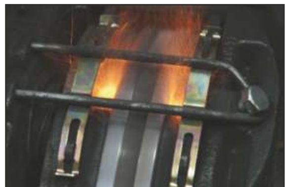
Brake disc under going thermal fatigue test
