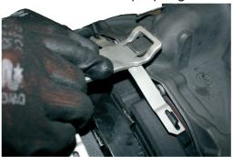
6. Press down on Retaining Bar and push in Retaining Pin
