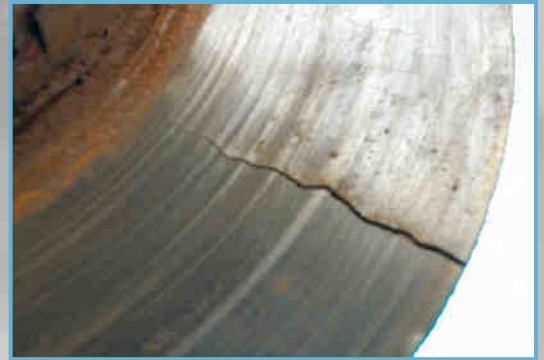
Image 1 - Cracked Disc Face
