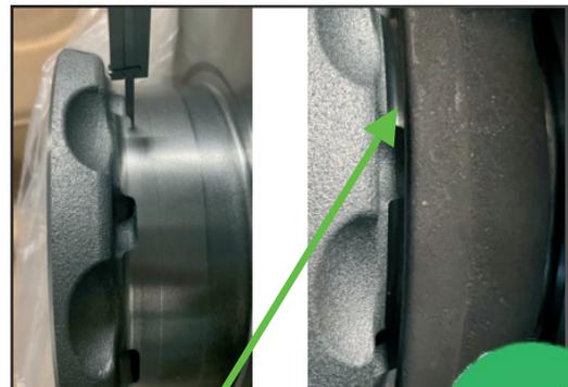
WINNARD Brake Disc does **NOT** contact the brake carrier.
