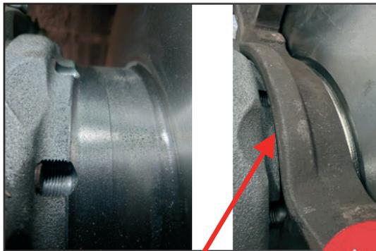
Brake Disc is in **contact** with carrier, creating noise, heat and wear issues.
